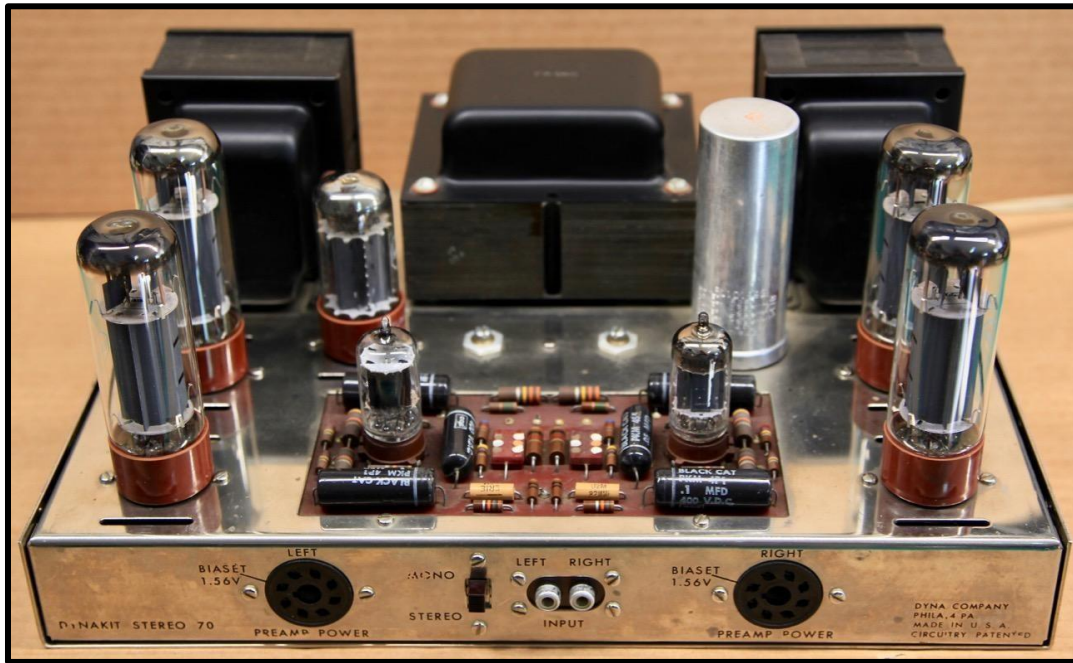
An Original ST-70 with a first-generation PA-060 Power Transformer
