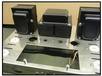
c- the remaining 'two holed' spacers get screwed into the top two holes of the cutout to the inside of the chassis, you should end up with four spacers on the inside and four spacers on the top of the chassis, see photo.
