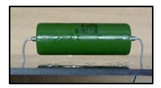
Other than the spacing for PIO coupling capacitors, assembly of the CCA is straight forward and simple. Use a capacitance meter and a digital VOM multimeter to ensure that all component values are verified before installing in the CCA. Again, we stress the importance of GOOD SOLDERING!
