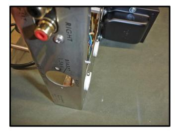
b- Two of 'two holed' spacers is screwed onto the threaded studs in the front holes and two in the rear holes using 4-40 screws, on the top of the chassis, see photo.
