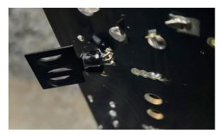
CCA, then trimming the lead excess from the top of the PC board.
