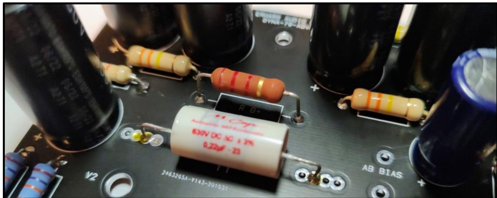
Photo 2: The 3 Watt B+ Resistor is Mounted 1/8 - 3/16 of an inch above PCB (Brown-Orange resistor in photo center)
