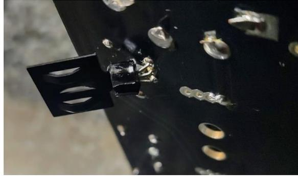
It's acceptable for the heat sink to touch the ST-70 chassis, but in no way should it ever be forced into place. Also ensure that the heat sink does not contact the solder points for R12. This was not an issue in our prototype development, but if not aligned properly, it could touch one of these R12 solder locations and ground the circuit through the heat sink to the chassis. Do Not Let the heat sink touch any electrical connection points.
