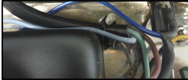
58. Route the power cord's black HOT/LIVE wire behind the power transformer and solder it to the bottom tab of the power switch. We recommend that you use heat shrink to insulate the joint.
