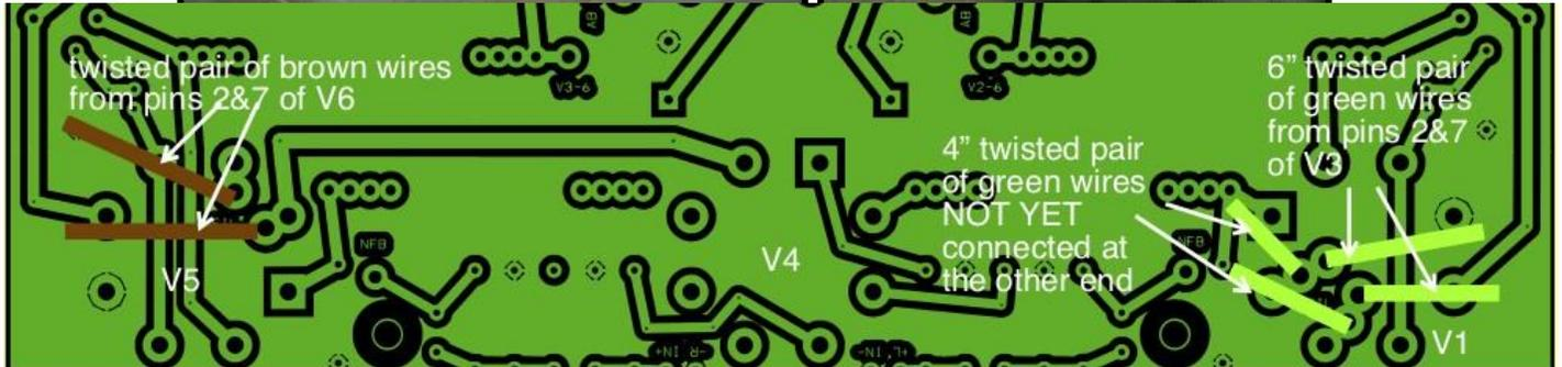
47. Speaker terminal connections (NOTE: If you did not remove the old Dynaco speaker terminals or any transformer wiring to them, skip this step).
