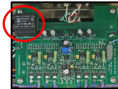
B- Second Generation Module w/ Transformer
